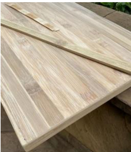
Fig16: Rice husk particle board with bamboo strips facing
