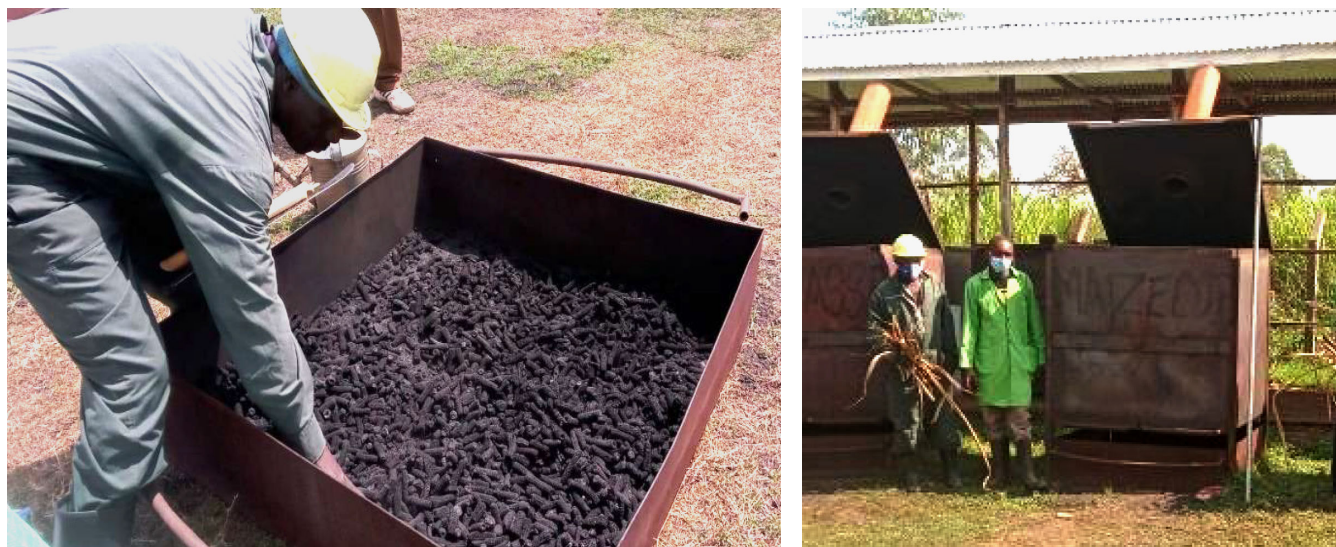
Fig17: Carbonization of maize cobs using the improved KEFRI's TLUD Box Kilns and (Right) carbonized maize cobs
