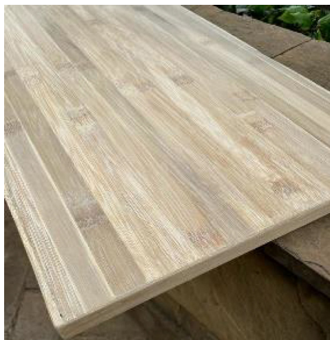
Fig16: Rice husk particle board with bamboo strips facing
